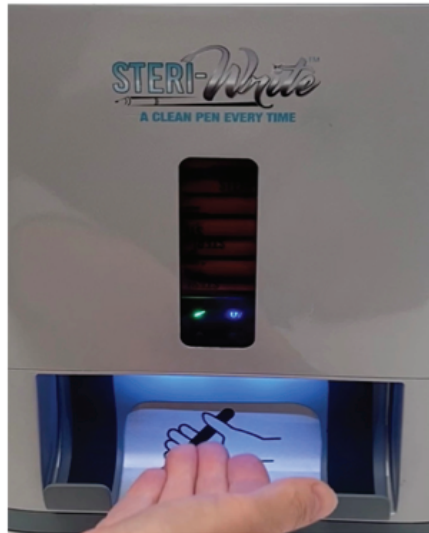
Figure 3. Visualization of how to summon a sanitized pen. There are touchless sensors within the illuminated area. Hand should be placed within this area to activate the sensors, but hand does not need to touch the Steri-Write™ device. A clean pen will drop into the cradle to be removed.
